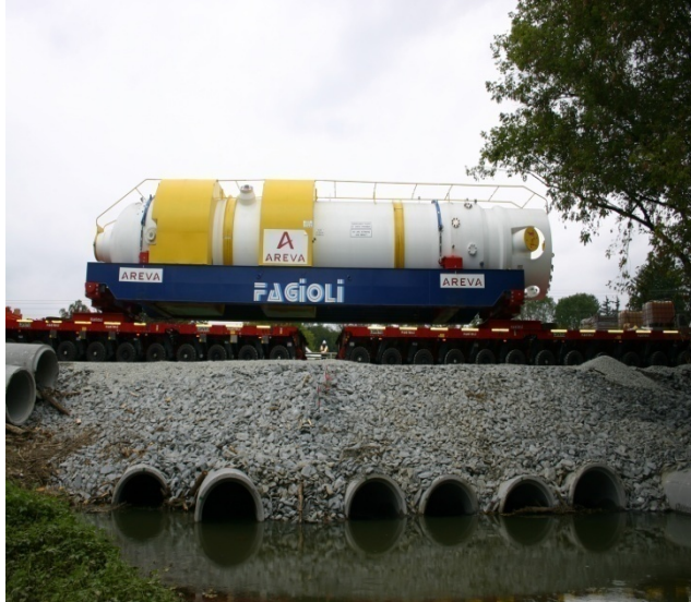
Just like a scene from the History Channel's "Mega Movers" Fagioli, Inc. of Houston, Texas and Areva NP Inc. Lynchburg Va. move two 510 ton steam generators to Exelon's TMI-Unit I Nuclear Power facility in Middletown PA.
