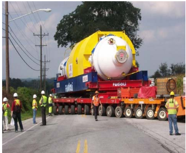
825 ton transport vehicles (26 axles and 208 wheels) and some the 100+ people that it took to make sure the move went off without a hitch.
