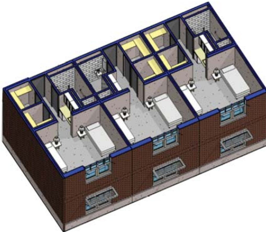
(2) Structural Precast Concrete Modules make up a single BEQ Room
